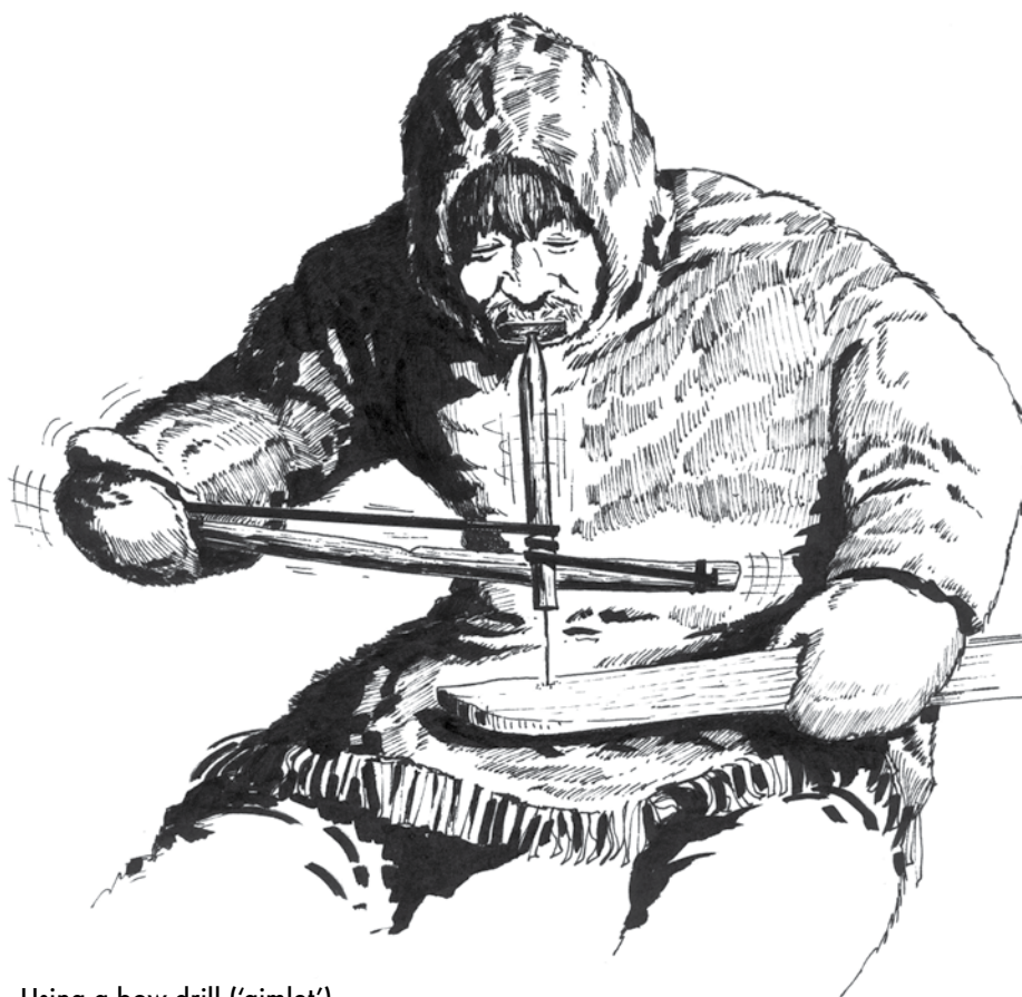
Using a bow drill ('gimlet').
