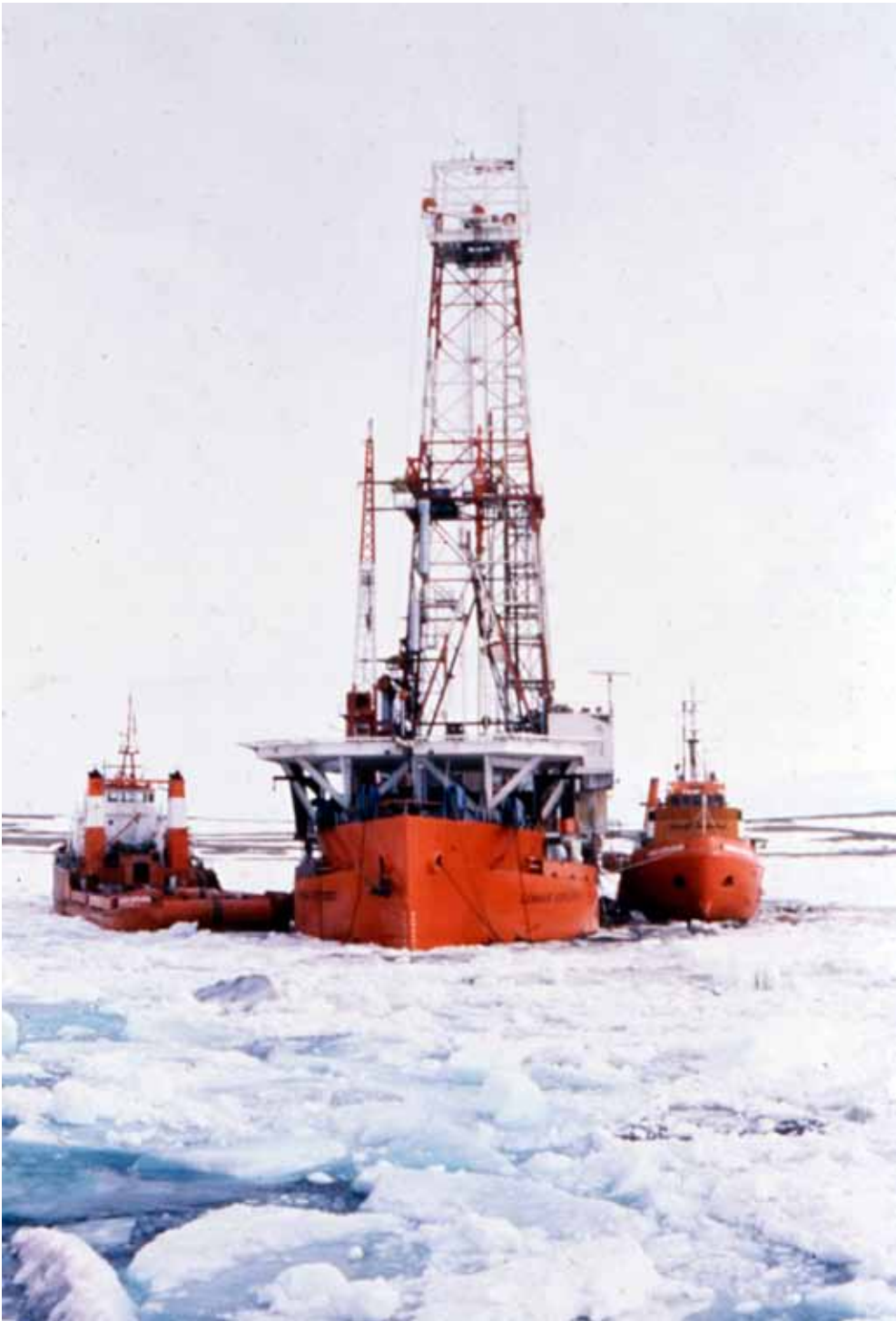
An ice-reinforced drill ship in the Beaufort Sea. (Chevron Canada)
