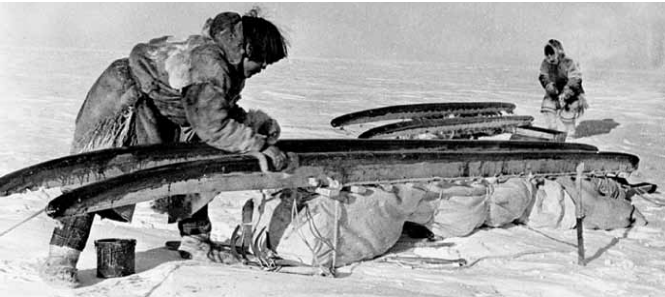
Moss and water are frozen onto the bottoms of sled runners to help them slide over the snow. (Fleming/NWT Archives/N-1979-050-1176)
